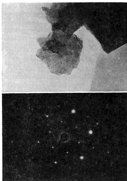
Fig. 5. Bright-field electron micrograph and selected area electron diffraction pattern of graphitic particle in the carbon specimen heat-treated at 1100°C for 60 min under 3.2 kbar in the presence of calcium oxide CaO-9.
